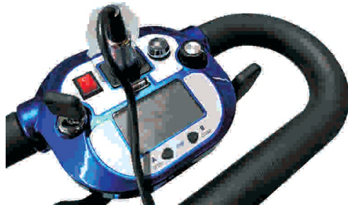
Insert charging plug into charging socket
