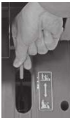
Disengage and in freewheel mode.
