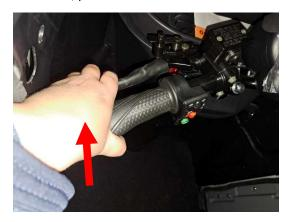
While still holding the brake, use your other (right) hand to press the click button down to lock it in! Once it is pushed down, hold, and let go of the brakes. They should stay in the locked position.
