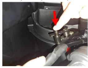
To release the brakes, simply grab the hand brake and squeeze. The click button will pop up when you release the lock lever.
