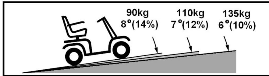
When driving up an incline, try to keep your scooter moving. If you must stop, start up again slowly, and then accelerate cautiously. When driving down an incline, set the speed switch to MIN and drive forward only. If your scooter starts to move down the incline faster than you want, allow it to come to a complete stop by releasing the throttle control lever, then push the throttle control lever forward slightly to ensure a safely controlled descent.
