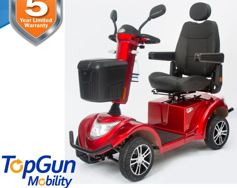
TG600RS Multi Terrain vehicle. With one of the most powerful motors and big 12" wheels it's born to run over ground without compromising on comfort. A cushioned captain style seat, armrest, headrest, pressure sensitive control panel and adjustable tiller are standard equipment. Can be operated with either right or left hand.
