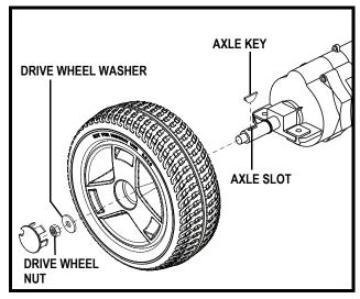
Figure 26. Solid Tyre Wheel Removal
