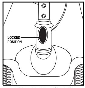
Figure 21. Tiller Lock knob (Locked)
