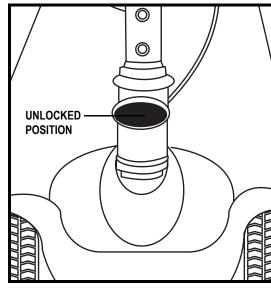
Figure 22. Tiller Lock Knob (Unlocked)
