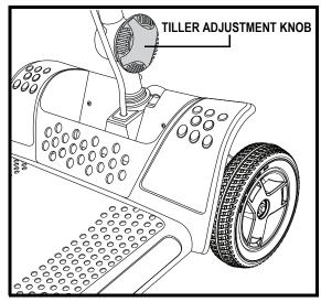
Figure 15. Tiller Adjustment Knob
