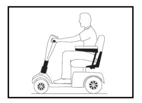
Figure B. Normal Driving Position
