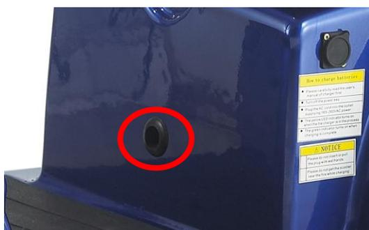
When the voltage in your scooter’s batteries becomes low or the scooter is heavily strained because of excessive loads or steep inclines, the main circuit breaker may trip to protect the motor and electronics from damage.
