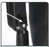
Reinforced armrest It allows for the additional stress of getting on and off the Comet HD.
