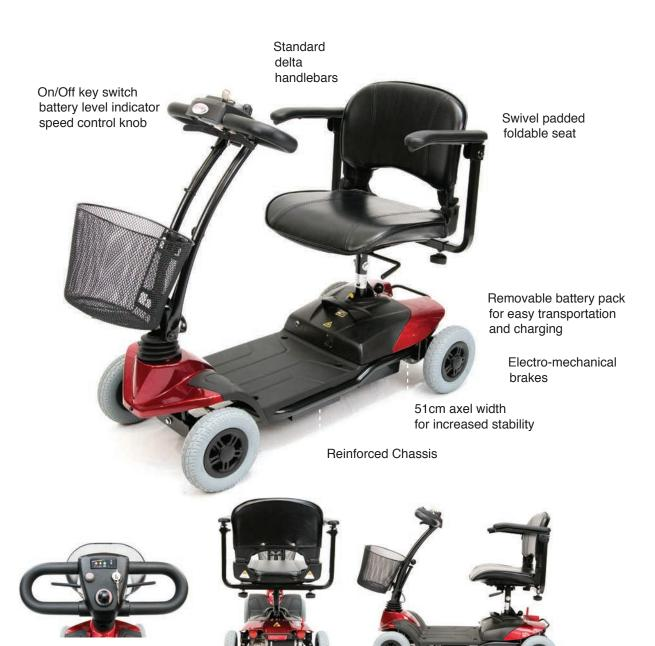
**Overall Height:** 89cm **Overall Length:** 100cm **Overall Width: 52cm** Weight with battery: 40kg
