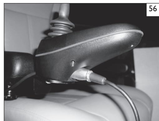
Off-board charger port located under joystick
