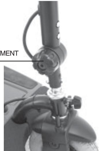
FIGURE 12. TILLER ADJUSTMENT
