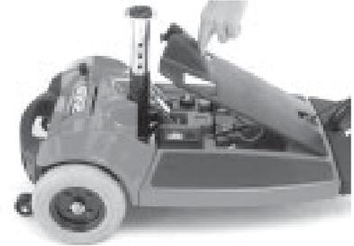
FIGURE 10. BATTERY COMPARTMENT LID
