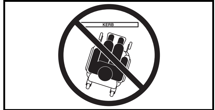
Figure 3. Incorrect Kerb Approach
