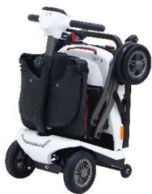
Automatic folding by pressing remote control.
