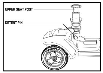
Figure 17. Seat Height Adjustment
