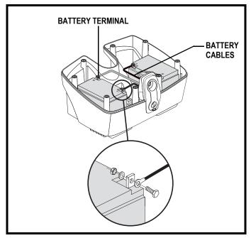
Figure 14. Battery Replacement
