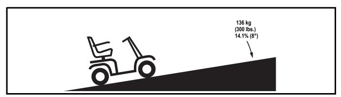
Figure 1. Maximum Recommended Incline Angle
