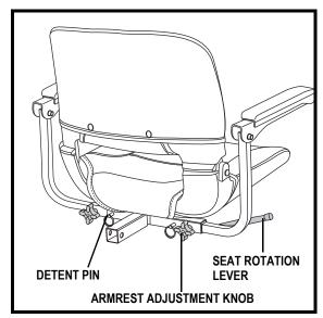
Figure 16. Seat Adjustments
