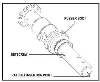
Figure 18. Seat Suspension Adjustment
