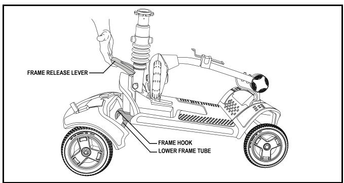
Figure 23. Frame Release Lever
