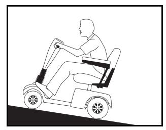
Figure 2A. Increased Stability Driving Position
