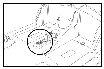
Figure 8. 3-amp Tiller Console Fuse
