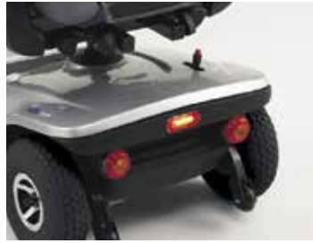
Rear brake lighting warns other people that the scooter is slowing down, thus preventing collisions.
