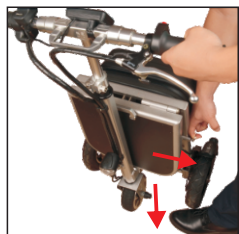
4. Place your foot before rear wheel and pull the folding lock.
