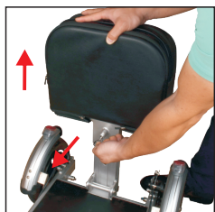
8. Pull the zipper and pull the seat upwards
