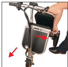
5. Pull the folding lock and handlebar spreads forward
