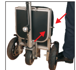
9. Pull hard and you would hear the clicking sound.
