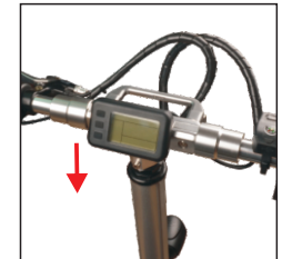
6. Pull the headstock downwards
