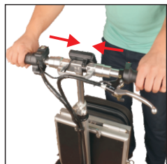
3. Pull up, hear the sound, the Lock sleeve is locked.
