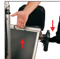
8. Tighten the rear wheels with one foot
