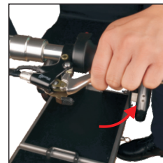
1. Hold the brake handle.
