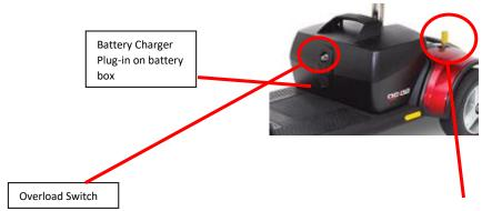
If all the power from your mobility scooter "cuts out" [the scooter doesn't go, the lights for the battery indicator don't turn on, the horn doesn't work, it becomes "dead"], check if the overload switch has popped out on the battery box.
