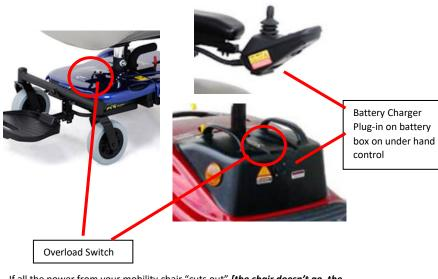
If all the power from your mobility chair "cuts out" [the chair doesn't go, the lights for the battery indicator don't turn on, the horn doesn't work, it becomes "dead"], check if the overload switch has popped out on the battery box.
