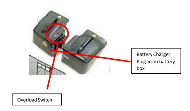
If all the power from your mobility scooter "cuts out" [the scooter doesn't go, the lights for the battery indicator don't turn on, the horn doesn't work, it becomes "dead"], check if the overload switch has popped out on the battery hox
